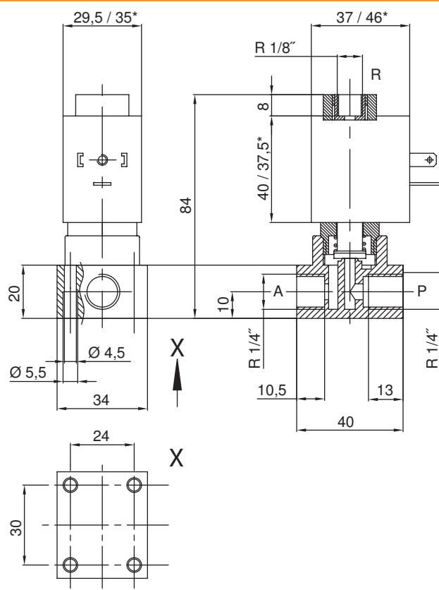
The ventilation connection R can be fitted with a sintered bronze silencer R 1/8" (Art.-No. 215/000011) as ventilation filter.
