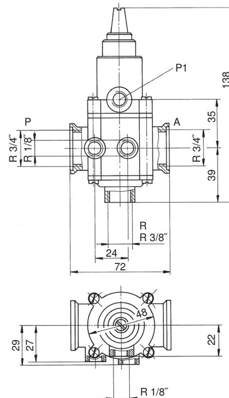
Connection R 1/8" are fitted with screw plugs as standard.
